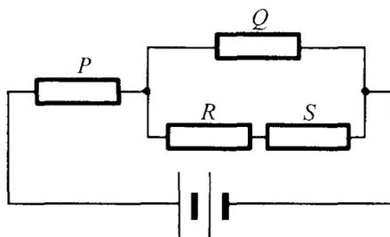
If the power dissipated by  $R$  is 1 W, find the total power output of the battery.
