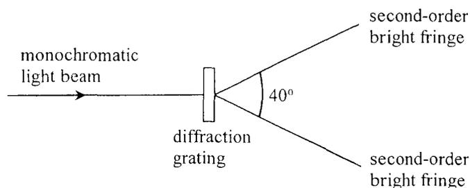
When a monochromatic light beam is incident normally on a diffraction grating with 300 lines per mm, a pattern of bright fringes is formed. The angle between the two second-order bright fringes is  $40^\circ$ . Find the frequency of the light.
