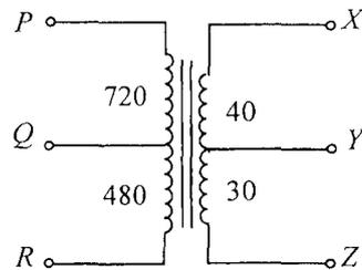
The above figure represents a multi-tapped transformer. The number of turns between the various 'tapping points' are indicated as shown. Which connections should be used for stepping down a voltage from 240 V to 6 V ?
